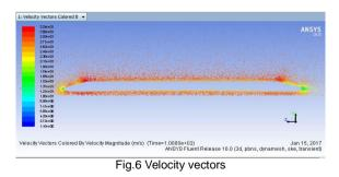
As we can see from the above fig. the maximum velocity vectors at both head and it is recognizing by red color where as minimum is blue color. Velocity vectors are denoted by an arrow.
